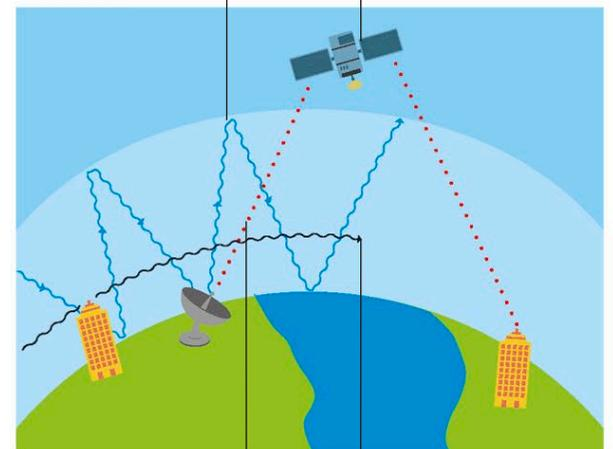
High-frequency signals pass through the ionosphere to reach satellites.
