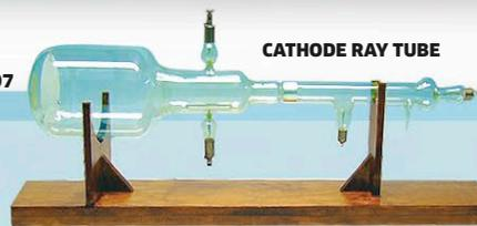
**CATHODE RAY TUBE****Discovery of electrons**
