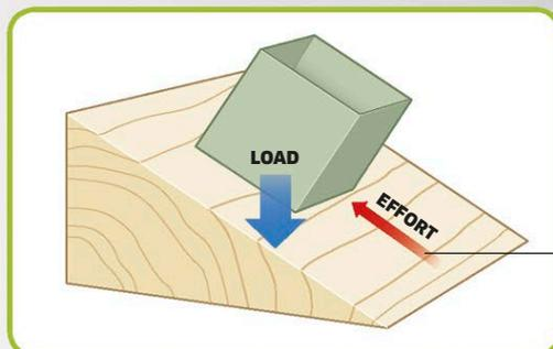
Less effort is needed to push a load up a ramp, but the load has to move further along the slope than it moves vertically.
