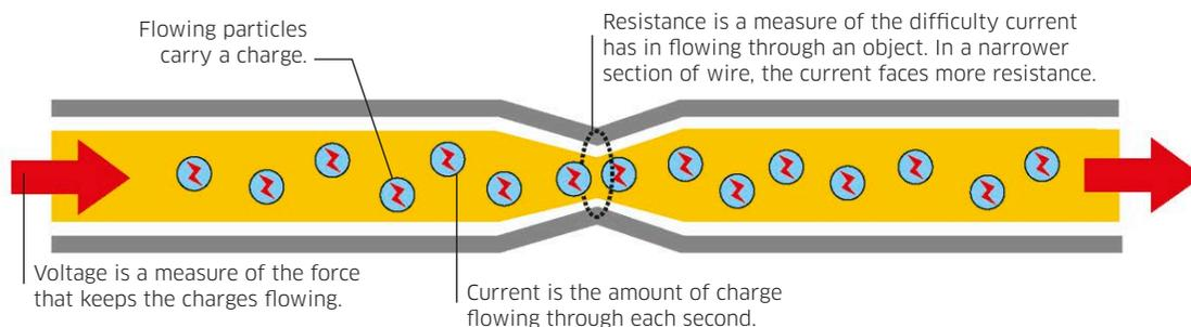
$$\text{Resistance in ohms} = \frac{\text{Potential difference in volts}}{\text{Current in amperes}}$$
