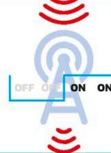
**2** The 1s and 0s of the binary number 0011 become off/off/on/on. The phone transmits the on/off values, encoding them as sudden changes to the signal's waves. The signal passes from base station to mobile exchange to base station.
