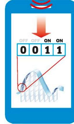
**3** The phone receives the digital signal and interprets the on/off transmission as strings of binary numbers. The phone's digital to analog converter turns the binary numbers back into analog information.
